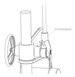
(pos. 2) lightly greased and clean. Dirt or damage to the toothing of the toothed rack must be avoided at all costs, as this may cause further damage to the pinion shaft (Pos.3) and impair or make impossible the further operation of the press.
